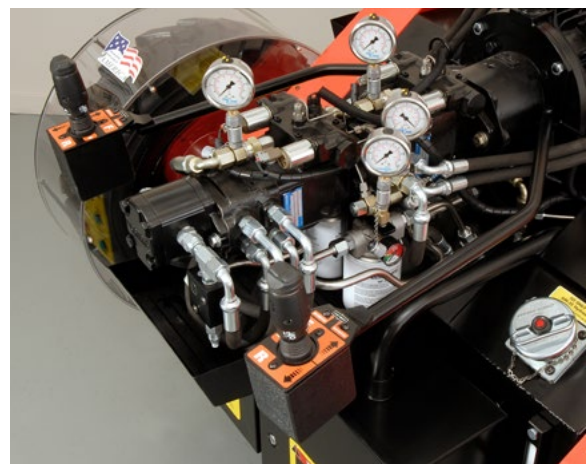
Dual tandem-pumps with dual joysticks and electronic pump displacement controls
