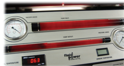
Transparent, back-lit suction & pressure lines
